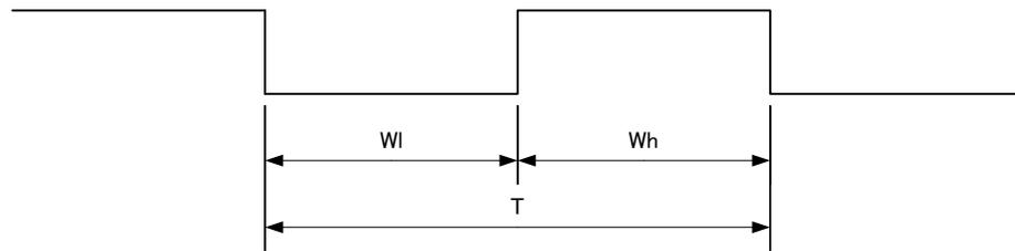
$$T = (\text{CmpB} + 1) \times \frac{1}{\text{CLK}} \quad (\text{S}) \quad \text{Wi} : \text{Wh} = \text{CmpA} + 1 : \text{CmpB} - \text{CmpA}$$
